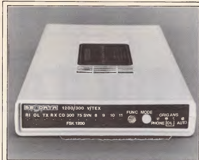
Australian modem manufacturer, Sendata, has produced an 'all-in-one' unit. It's capable of 1200/1200, 300/300 and 1200/75 baud and has auto answer and disconnect facility; but all this doesn't come particularly cheap at $1,300.
